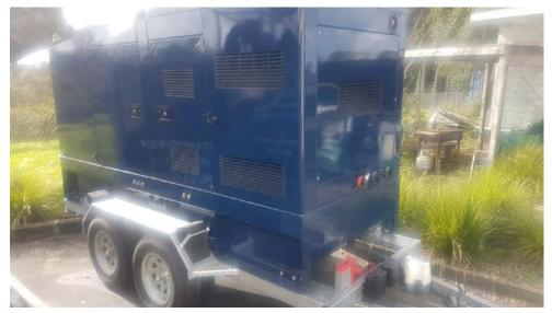
200kVA trailer mounted mobile generator (not branded)
