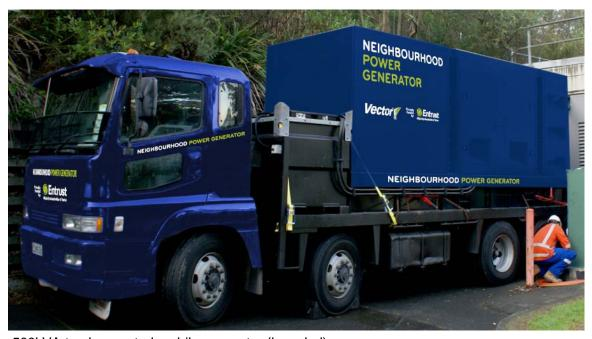
500kVA truck mounted mobile generator (branded)
